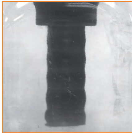
AFTER: once the magnets have been introduced, the entire magnetite sludge is quickly bound and can be flushed.
