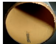
3" Copper Pipe - Covered with physical impurities*
